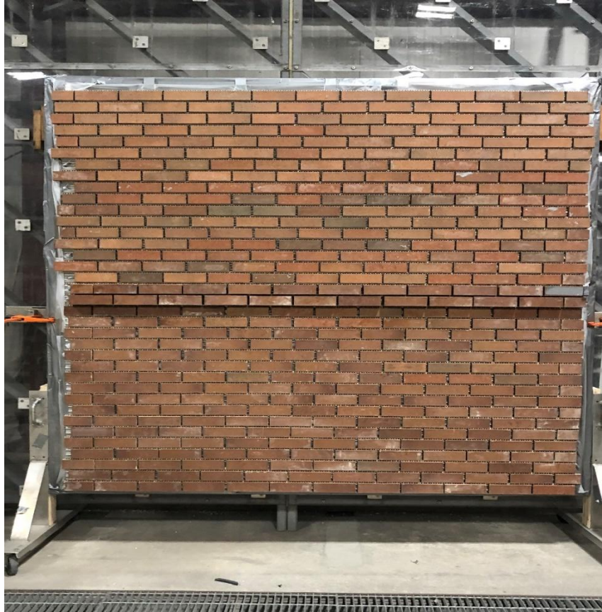
Photo No. 1 Brick Rainscreen System (without mortar)
